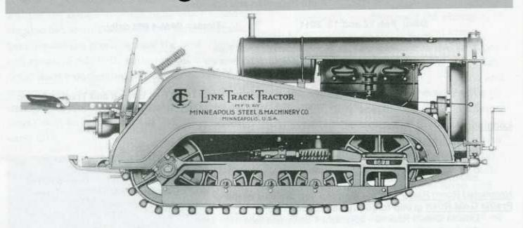
Drawings of a crawler tractor based on Twin City 12-20 tractor components have been known to exist for many decades. The popular black and white Twin City Photo Archive book, released in 1993 and edited by Peter Letourneau, contained these drawings of a small track equipped Twin City 12-20 labeled Link Track Tractor.
